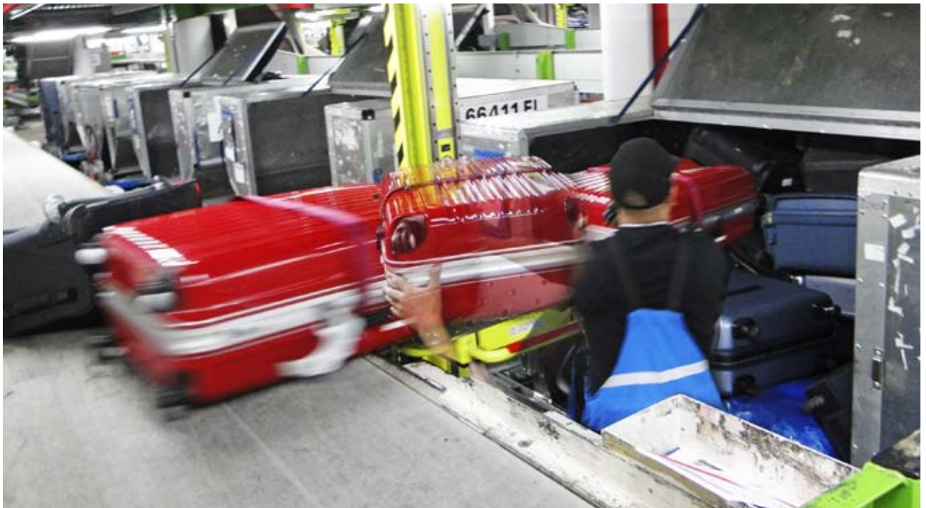
A specific lifting aid for loading and unloading containers was nowhere to be found, until the Container Loading System (CLS) was developed.
